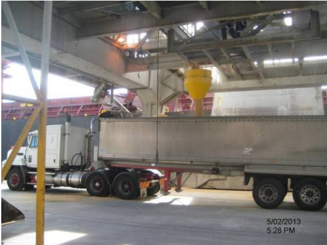
Figure 4 Un-loader A DSH Hopper in operation loading truck after further adjustments.
