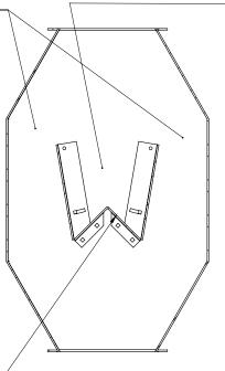
Angled center baffle aids in clearing the cushion pocket when adjustable baffels are set for self cleaning
