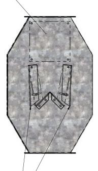
Adjustable baffles to allow for self-cleaning in full flow applications and for total flow restriction in low flow applications to ensure grain quality.
